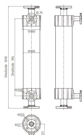
Dimensions apply to ABS Shell material.
