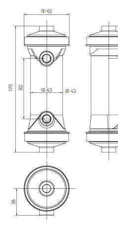
Dimensions apply to PSU Shell material.
