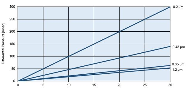
Water Flow Rate at 20 °C [L/min] 10" cartridge
