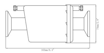
Inlet/Outlet: 38 mm (11/2") Sanitary flange
