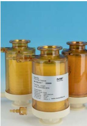
The **MasterSip MS-Capsules** are designed for use in sterile air and gas filtration in biopharmaceutical and other applications. Composed of a hydrophobic 0.2 µm PTFE membrane and a polyetherimide housing, these capsule filters provide an alternative to a stainless-steel housing/filter combination and thus reduces operating costs and maintenance time.
