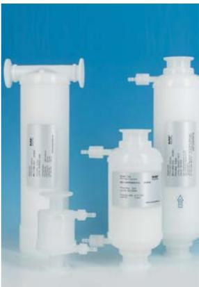
The **MasterCap MC-Capsule** are used for removal of micro-organisms and fine particles from liquids and gases. Made of polypropylene shell and high-performance filtration media such as PP, PES, PTFE, PVDF, NYLON and Glass Fiber (GF) with a pore size of from 0.1 to 10 µm. They are the ideal filters to satisfy the highest standards in a broad range of applications.
